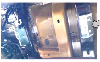
6. Place M8 cage nuts on the inside of the canister brackets as shown. Attach to vehicle using factory hardware as shown.
