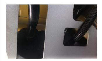
14. Replace canister hoses as shown. Check clips have secured correctly by gently pulling hoses towards rear of vehicle.
