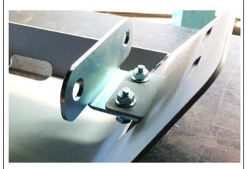
8. Install canister bracket to canister panel using M8 x 25 mm bolts, flat and spring washers, as shown, finger tight only.
