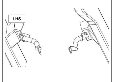
18. Fit left and right braces to the underside of engine mount brackets as shown. Fasten using M10 bolts, spring washers, flat washers and M10 flange nuts finger tight only.
