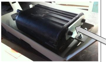
11. While firmly pushing the rear canister bracket on to the canisters plugs in the direction shown, tighten the M8 bolts fitted previously.
