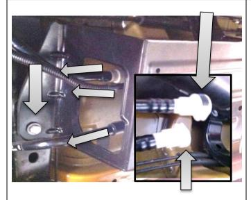
Remove the three hoses from the charcoal canister (rear LH side of vehicle) by pushing the tabs marked and removing to the rear of the vehicle.
