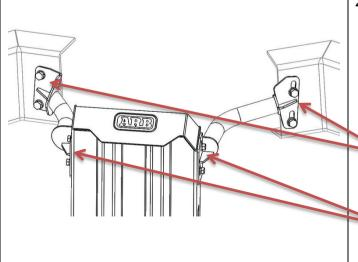
23. Adjust the front panel to the centre location, ensuring that a minimum 10 mm clearance is achieved from all engine components and piping.
