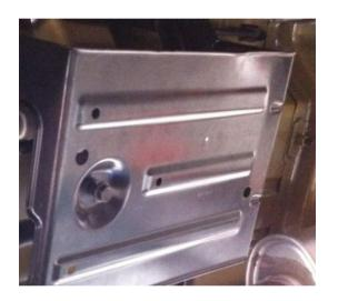
4. Remove and discard the bolt retaining the rear of the canister. Carefully remove and retain the canister.
