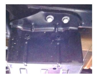
Remove and retain the remaining two bolts securing the front of the canister bracket.
